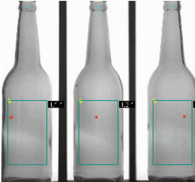
Resulting image with test contamination spots and overlaid detection graphics produced by the image processing software.
