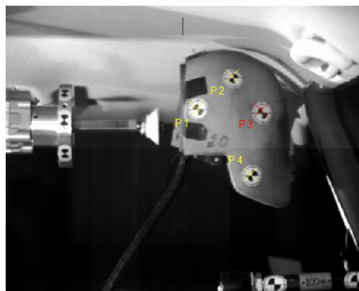
Analysing the 6DOF motion of a dummy head
