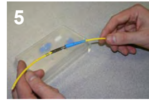
4 Slide cordage fiber through connector parts inside of packaging.
