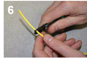
5 Remove cordage with connector parts attached.
