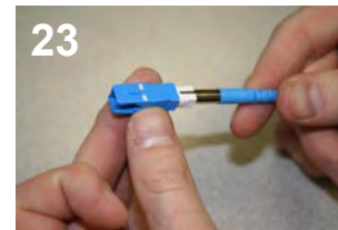
23 Slide outer housing over inner housing. Inner housing is keyed to outer housing.
