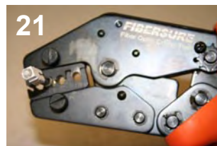
21 Crimp "sleeve" onto "crimp ring" using 0.178 hex slot.
