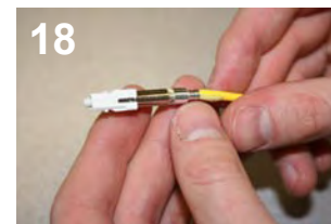
18 Slide up "crimp sleeve" so that the kevlar is pinched between crimp sleeve and main body.
