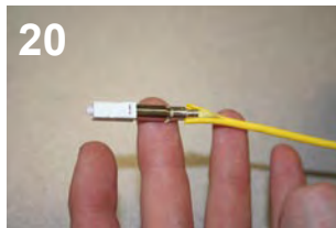
20 Remove split cordage from underneath "crimp ring."
