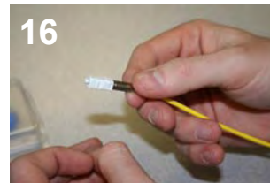
16 Place inner housing over main body and ferrule (for APC align dot with round side of inner housing). Stop ring is keyed to inner housing.
