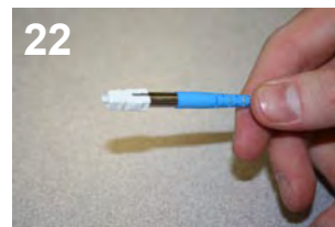
22 Slide boot over components. Main body is keyed allowing for boot to rest in proper position.
