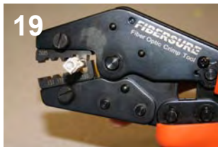
19 Crimp "crimp ring" onto main body using 0.190 round.
