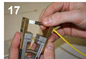
17 Use Connector Assembling Tool to snap on inner housing to main body.
