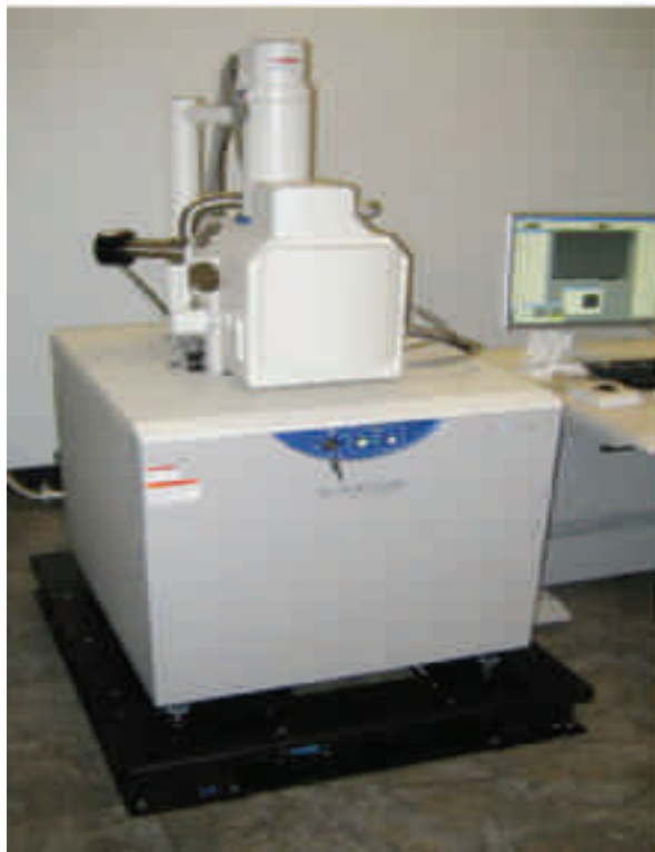
STACIS® iX SEM-Base™ Floor Platform isolating an FEI Helios NanoLab DualBeam SEM/FIB (top left), a JEOL JSM-6700F Field Emission Scanning Electron Microscope (top right), an Hitachi S-3400N SEM (bottom left), and a Zeiss UltraPlus Field Emission Scanning Electron Microscope (bottom right).
