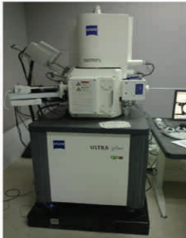
STACIS® iX SEM-Base™ Floor Platform isolating an FEI Helios NanoLab DualBeam SEM/FIB (top left), a JEOL JSM-6700F Field Emission Scanning Electron Microscope (top right), an Hitachi S-3400N SEM (bottom left), and a Zeiss UltraPlus Field Emission Scanning Electron Microscope (bottom right).
