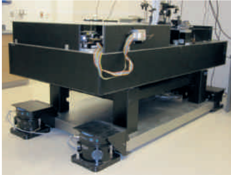
Until recently, researchers desiring the quietest possible vibration environment in a lab combined two independent products into a two-stage isolation system. This photo shows a 784 Series CleanTop® Optical Top supported by Gimbal Piston™ Air Isolators. This air isolation system is, in turn, supported on a 65 Series Floor Platform cradled with STACIS® 2100 Isolators. LaserTable-Base™ now combines these two independent isolators into one, integrated system.
