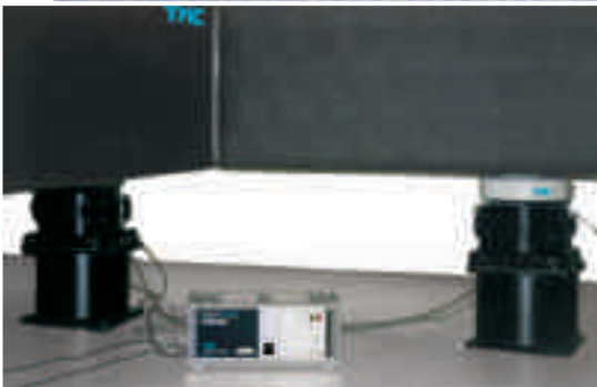
This eight-piece CleanTop® Optical Table System is installed at the Max Planck Institute in Heidelberg, Germany. The system may be configured as one entire assembly or smaller assemblies of one or more table units. The entire system is installed on a STACIS® Active Piezoelectric Vibration Cancellation System.
