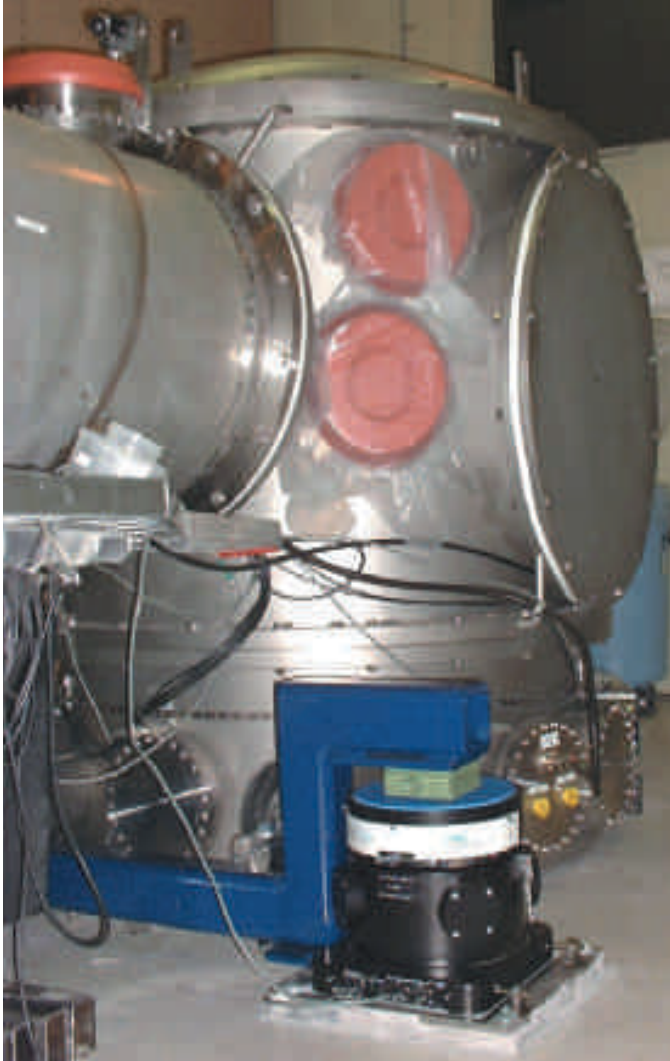
STACIS® supporting the end chambers of a prototype LIGO interferometer at the California Institute of Technology. These are the most precise instruments ever made – capable of measuring distances of less than 10^{-18} meters.
