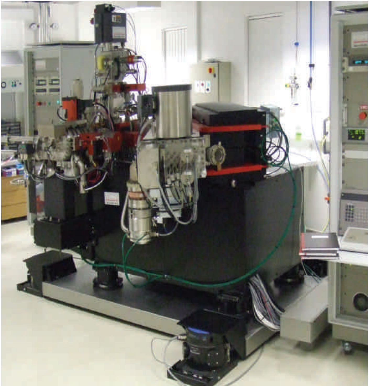
A Cameca NanoSIMS 50L on a TMC 65 Series Floor Platform supported by STACIS® isolators. This tool is a 5,000-pound secondary ion mass spectrometer with a spatial resolution of 50 nanometers. Photo courtesy of the Planetary and Space Sciences Research Institute (PSSRI) at The Open University, Milton Keynes, U.K.
